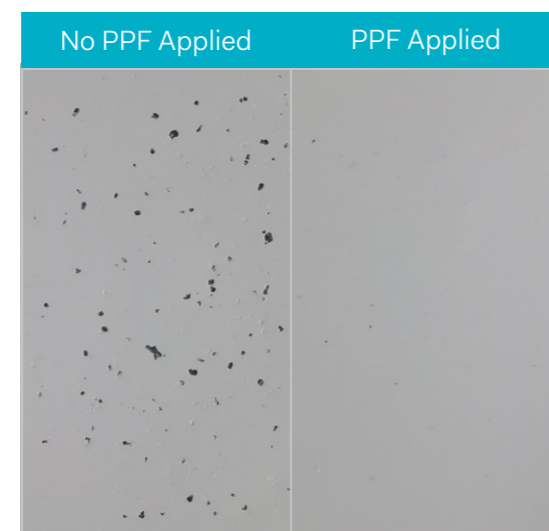
Image represents gravel impact testing on surface paint.
